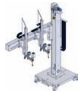
Station configuration 3 Side-boom manipulator with horizontally fixed boom, supporting one or two welding heads. This welding station, which offers flexible movement, is the basic unit for welding girders and profiles, and for joining plates and sections.
