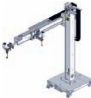
Station configuration 2 Conventional column-and-boom, with a movable boom and one welding head at boom end, combined with a boom-carriage-mounted welding head (not CaB 300).
