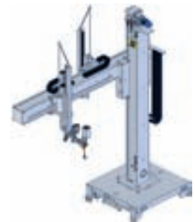
Station configuration 4 Side-boom manipulator with double-track boom. The welding heads are mounted either side of the boom. The boom carriages can be individually controlled by the joint tracking systems, on separate tracks. The welding motion from the rail carriage ensures a highly efficient welding process. Ideal for transversal double-fillet welding of stiffeners.
