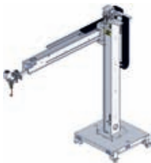
Station configuration 1 Conventional column-and-boom, with a movable boom, and welding head at boom end. Welding equipment can be positioned along four axes.
